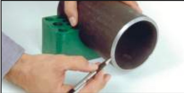
Step 1: Cut pipe end square, and bevel for butt weld.
