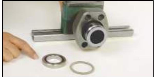
Step 2: Slip flange onto the pipe.
