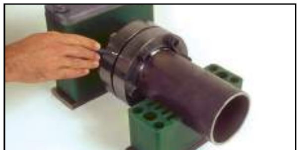
Step 6: Tighten bolts to the torque values specified. Always tighten bolts in a cross-over sequence and ensure the flanges are parallel.
