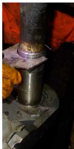
Crimping Diameter and Insertion Depth Verification
