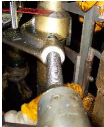
Cutting of Tube using Pneumatic Reciprocating Saw
