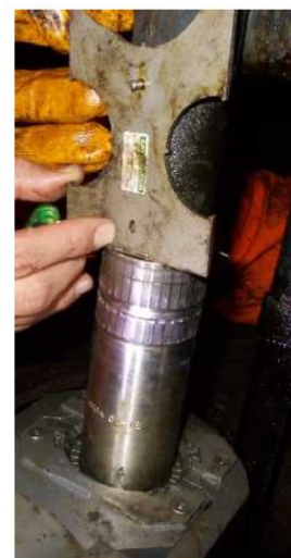
Crimping Diameter and Insertion Depth Verification
