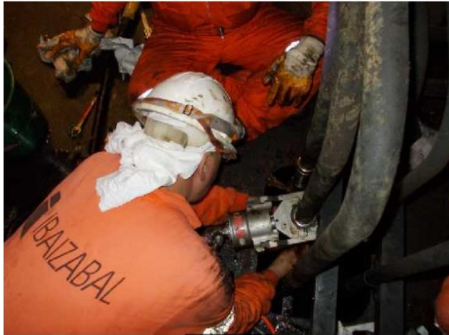
Crimping and inspection in any position
